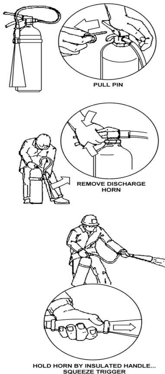
Figure 18-3 Operating the CO2 Extinguisher
